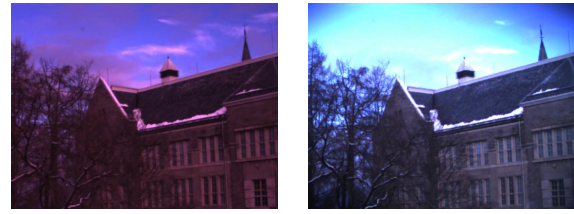
(a) Without UV/IR filter, 0.3 ms exposure time. (b) With UV/IR filter, 1.0 ms exposure time.
