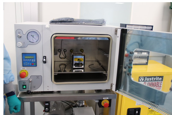
Fig. 6. FramSat-1 in a vacuum chamber prior to a test.
